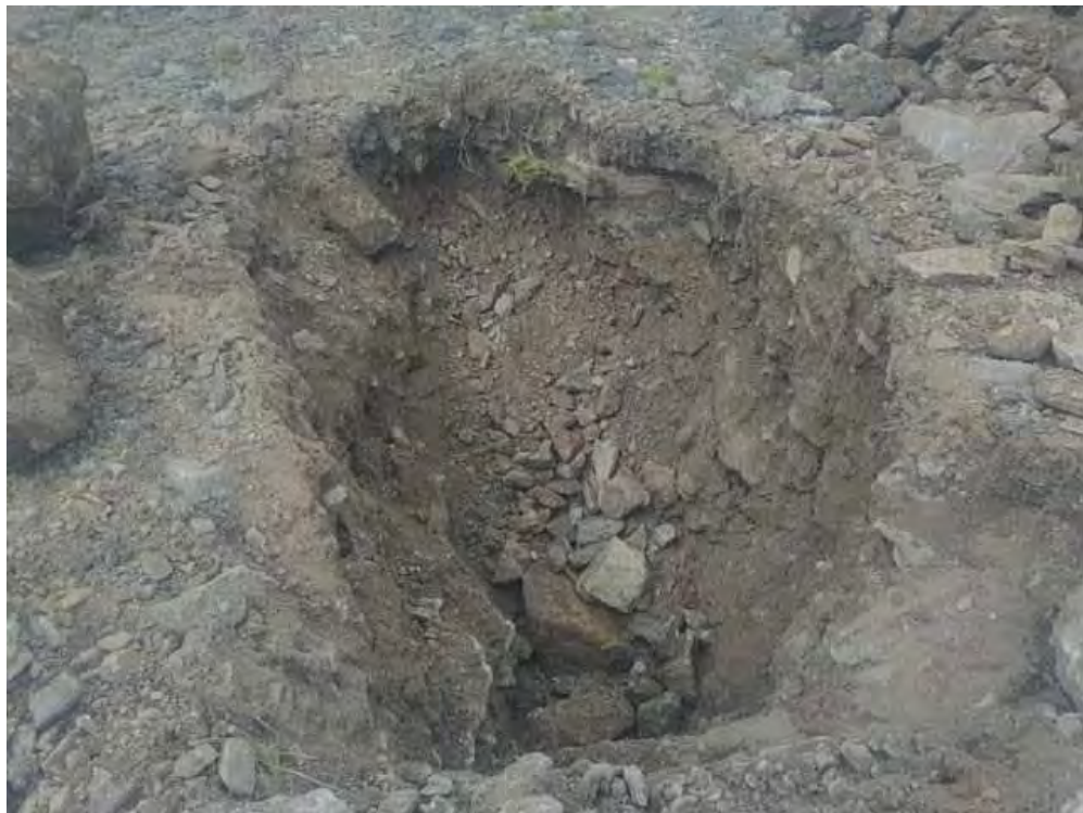
Photo 10. Test pit TP2, 0 - 1.0 mbgs (May 12, 2022).
