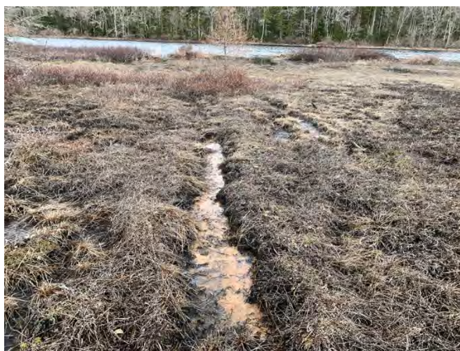
Photograph 6: View of well oxidized sandy tailings along the edge of the Tangier River
