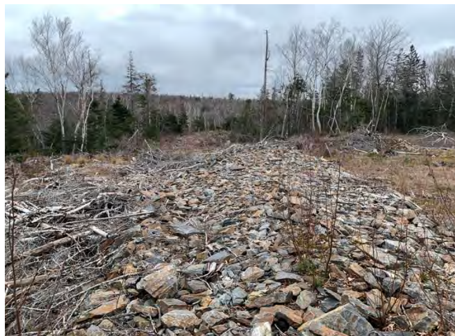
Photograph 2: View of oxidizing waste rock. Some vegetation present. Photo taken to the southeast of the area where the Quonset huts are located.
