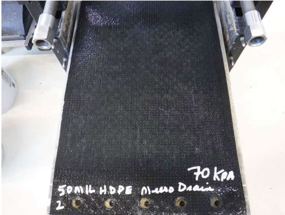
50 mil HDPE Microdrain Geomembrane after the test – Test at 70kPa
