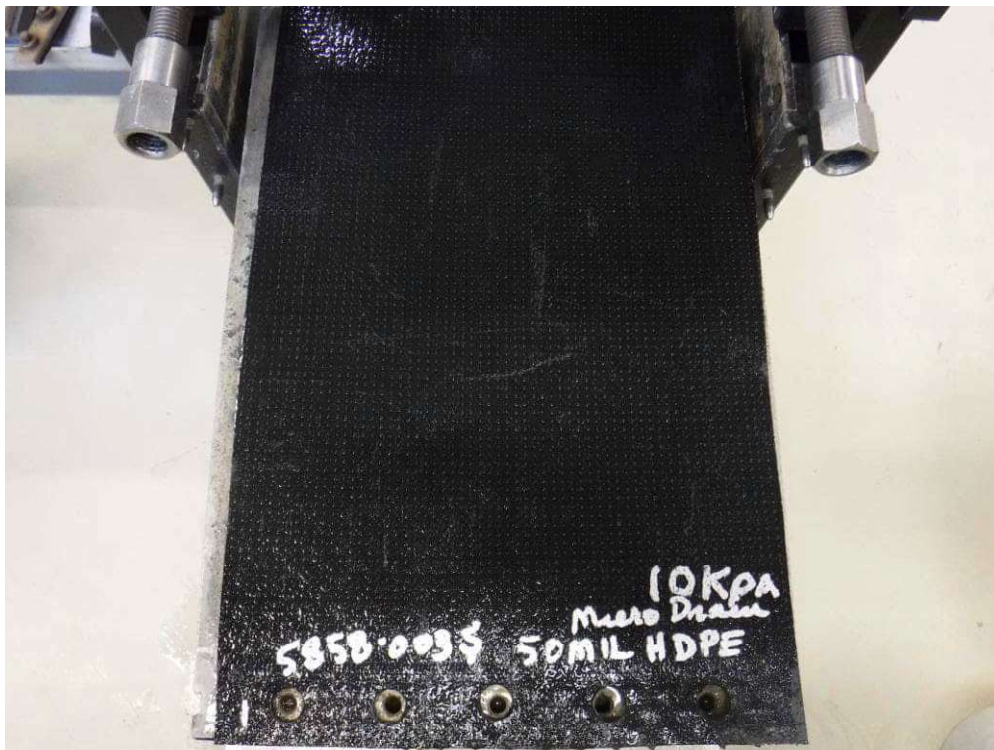
50 mil HDPE Microdrain Geomembrane after the test – Test at 10kPa
