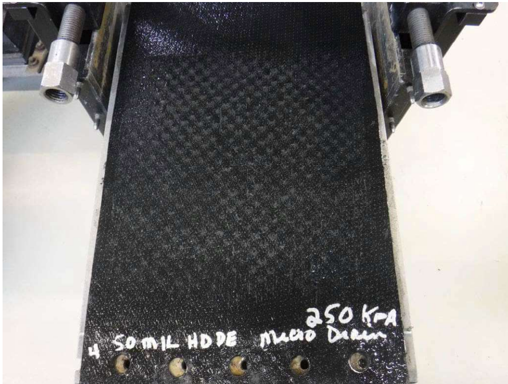
50 mil HDPE Microdrain Geomembrane after the test – Test at 250kPa
