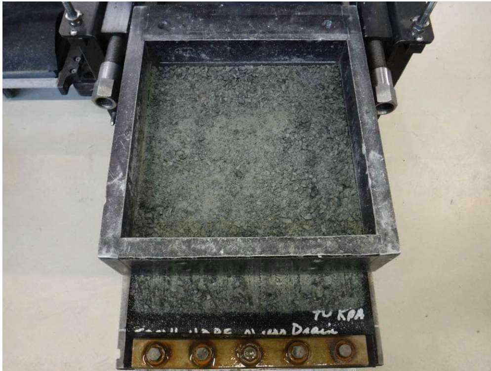
Soil (Crusher Dust “6mm minus”) after the test
