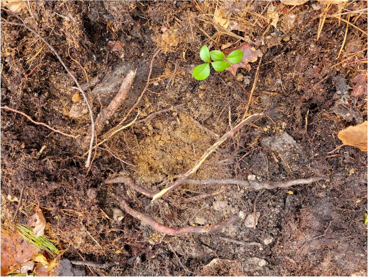
Figure 1: Soil Sample SS-1; Note presence of rocks and root mass.
