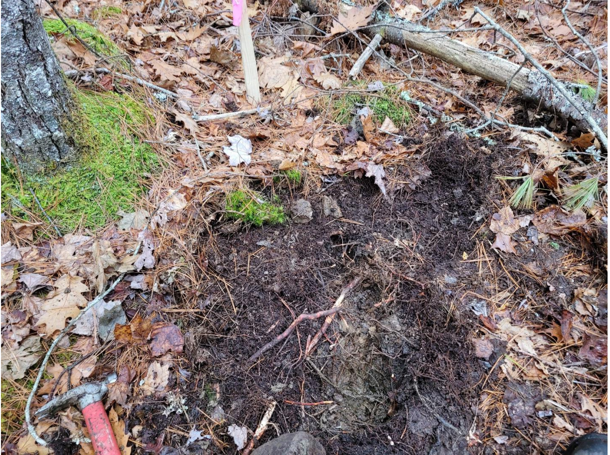
Figure 4: Soil Sample SS-11; note shallow depth of refusal.
