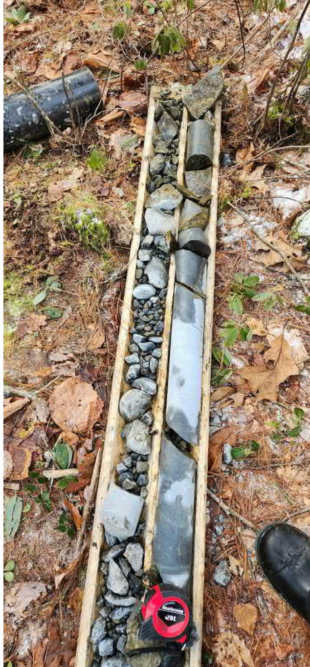
Photo 7: MW23-01, upper portion composed of boulders (left side with poor RQD) which transitions to competent bedrock (right side)
