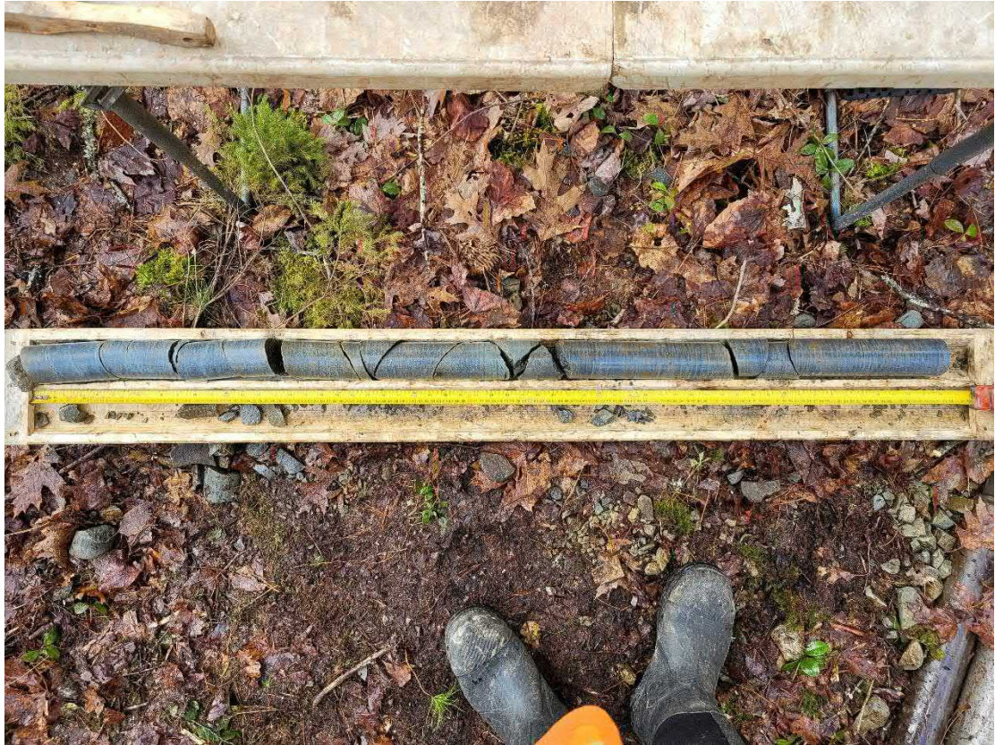
Photo 9: MW23-02, competent quartzite bedrock
