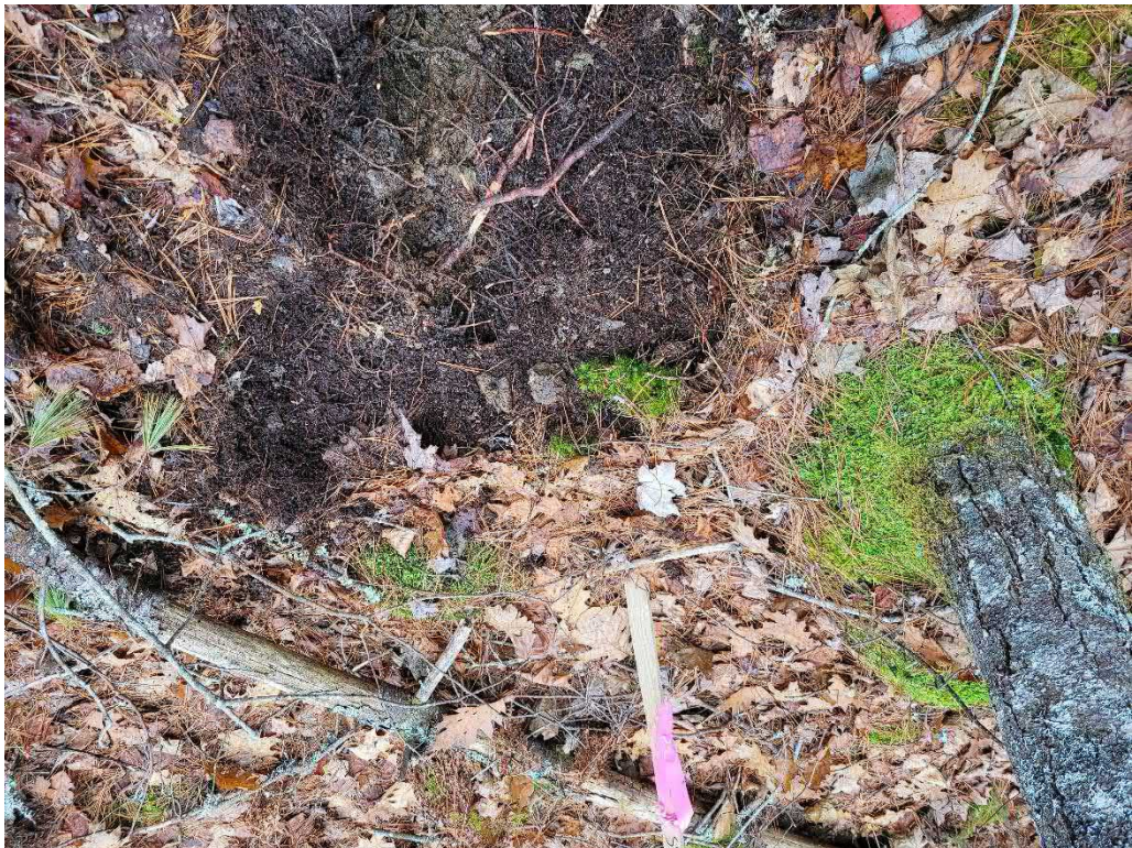
Photo 4: Soil Sample SS-11; note shallow depth of refusal.
